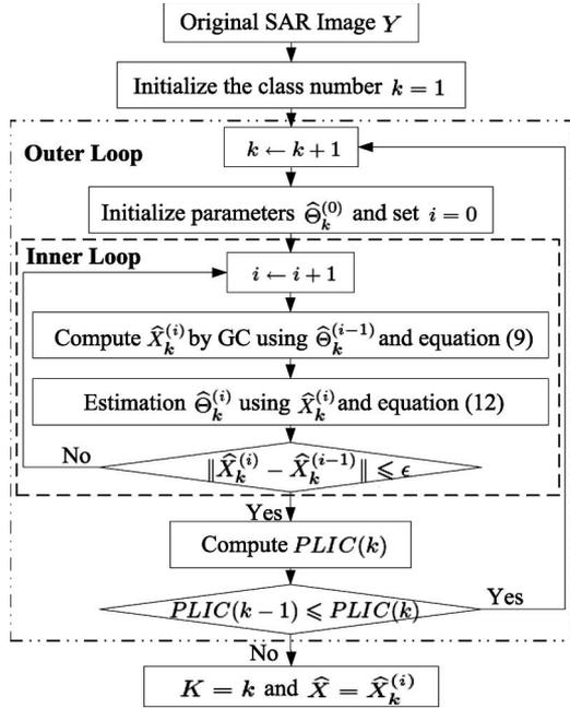
Fig. 1. Flowchart of the proposed RAMRF clustering method.
