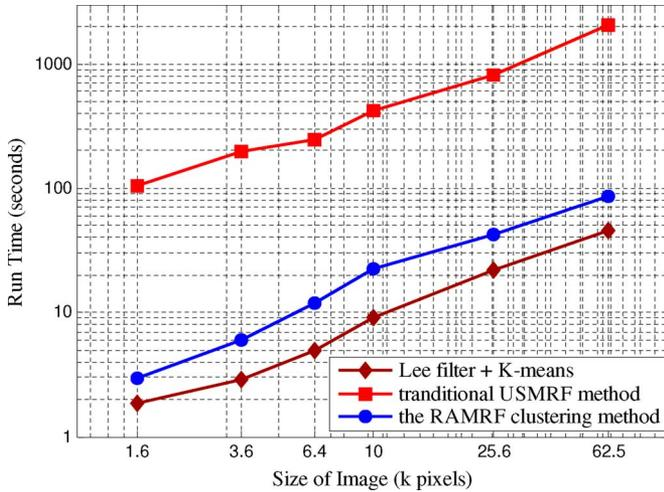
Fig. 4. Comparisons on running time. The three different methods are applied to different simulated SAR images with sizes of  $[40 \times 40, 60 \times 60, \dots, 250 \times 250]$ . The experiments are performed on a 2.8-GHz Pentium IV personal computer with 1-GB random access memory. We can see that the RAMRF performs faster than the traditional USMRF-based method but slower than K-means with Lee filtering beforehand.
