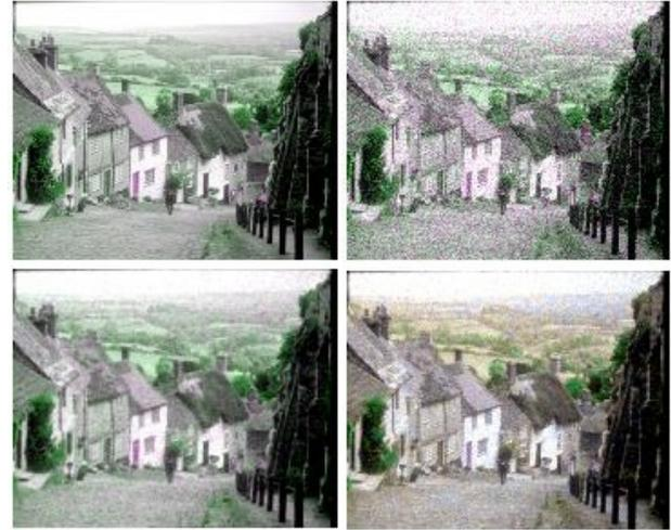
**Fig. 4.3.** Left Top : Ideal image, Right Top: add 10% speckle noise; Left Bottom : Refined Lee,  $SSIM = 0.7625$  , Right BottomOur result,  $SSIM = 0.7959$
