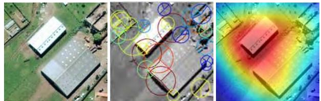
**Fig. 1: From left to right: a small GeoEye image containing buildings, junctions detected by ACJ, and computed PBI. The color indicates the significant level of buildings (red corresponds to high level).**
