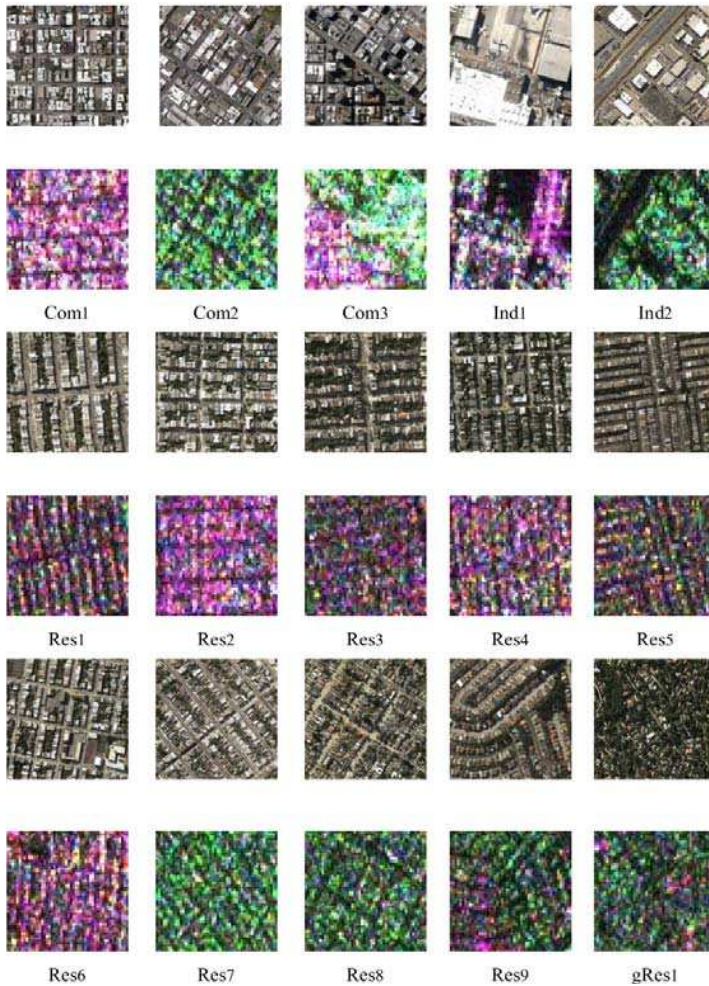
Figure 1. Samples of BAs in San Francisco. The lower row of each sample shows the PolSAR image, and the upper row shows the corresponding optical satellite images. Refer to the text for more details.
